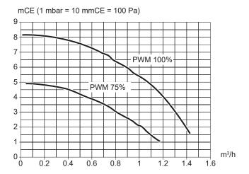
fig. 4 - Available hydraulic pressures and flow rates
