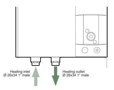
fig. 3 - Hydraulic connections
