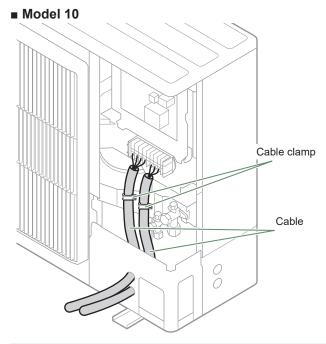
fig. 40 - Access to outdoor unit's terminal block
