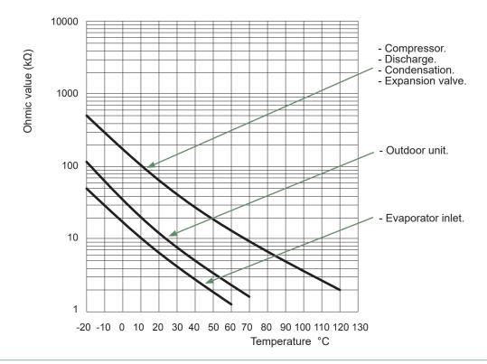
fig. 7 - Ohmic sensor values (Outdoor unit)
