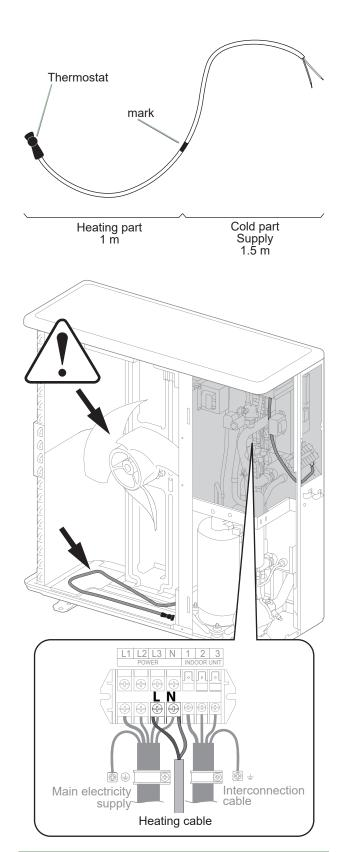
fig. 41 - Heating cable mounting
