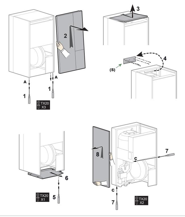
fig. 28 - Removing the casing
