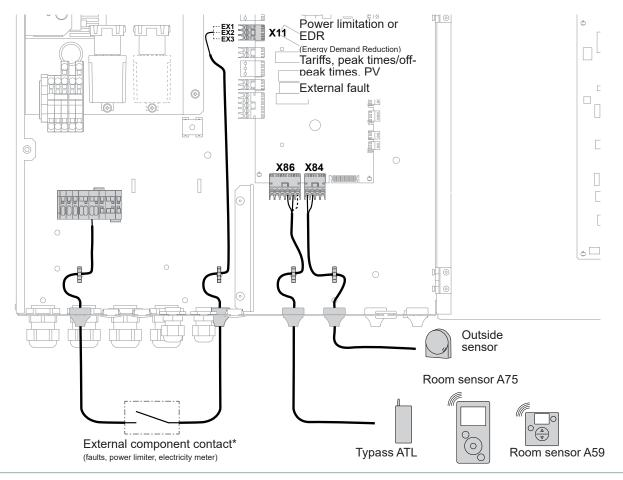
fig. 47 - Sensor cable feeds
