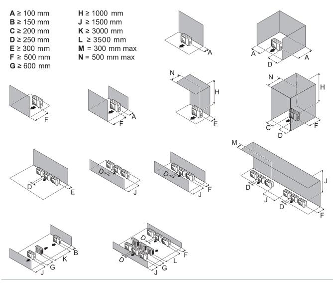
fig. 17 - Minimum installation clearances around the outdoor unit (model 10)
