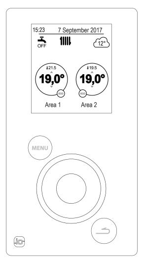
2 heating circuit version + domestic hot water (DHW)\*
