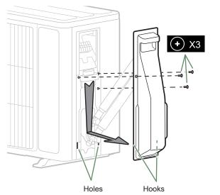
fig. 13 - Open the outdoor unit model 5, 6 & 8
