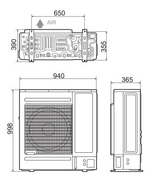
fig. 1 - Dimensions in mm
