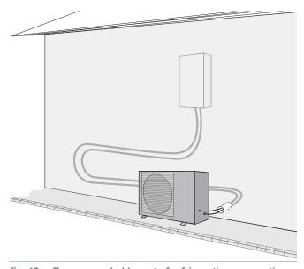
fig. 12 - Recommended layout of refrigeration connections
