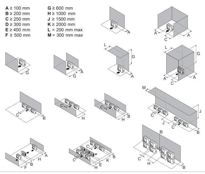
fig. 16 - Minimum installation clearances around the outdoor unit (model 5, 6 & 8)
