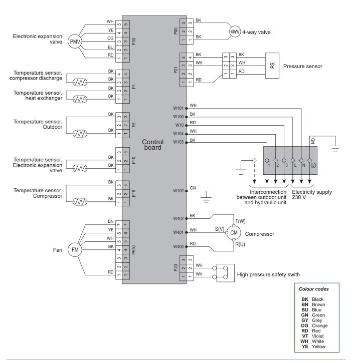
fig. 54 - Outdoor unit electrical cabling models 5, 6 and 8
