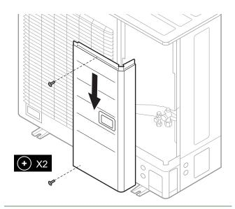
fig. 14 - Open the outdoor unit model 10
