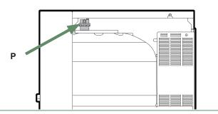
fig. 37 - Hydraulic unit automatic bleeder valve
