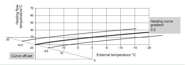
fig. 51 - Transferral of the heating curve
