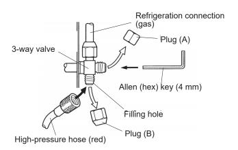
fig. 53 - Connecting the hose to the gas valve
