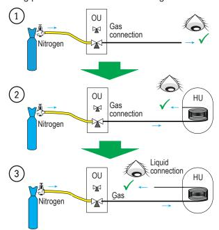
fig. 33 - Checking refrigeration connections
