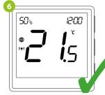
Both devices have been successfully linked. Thermostat displays the main screen, icon " $((\mathbf{P}))$ " appeared on the screen indicating connection with the receiver (ECB62ZB in this case).
