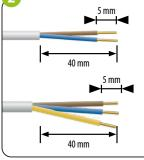
(min. 2 x 0,75 mm2 230 V max. 2 x 1.5 mm2 230 V) Power supply for the wiring centre, pump and 230V voltage
