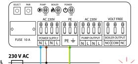
Power supply for wiring centre is  $230 \text{ V} \sim 50 \text{Hz}$ .
