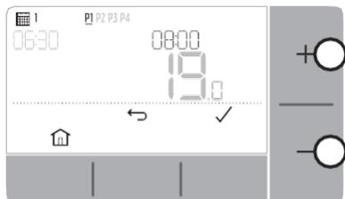
8. Press **←** or **→** to adjust the **temperature** and press **✓**
